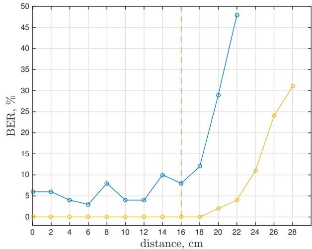
Fig. 7. BER depending on the distance from the point B. Area outside the laptop starts from 16cm. We use the following parameters: amplitude modulation (blue):  $t_0 = 0.5s$ , bitrate 2bit/s; periodic-based modulation (yellow):  $t_0 = 0.25s$ ,  $t = 15s$ ,  $p_0 = 3$ ,  $p_1 = 5$ , bitrate 0.067bit/s.
