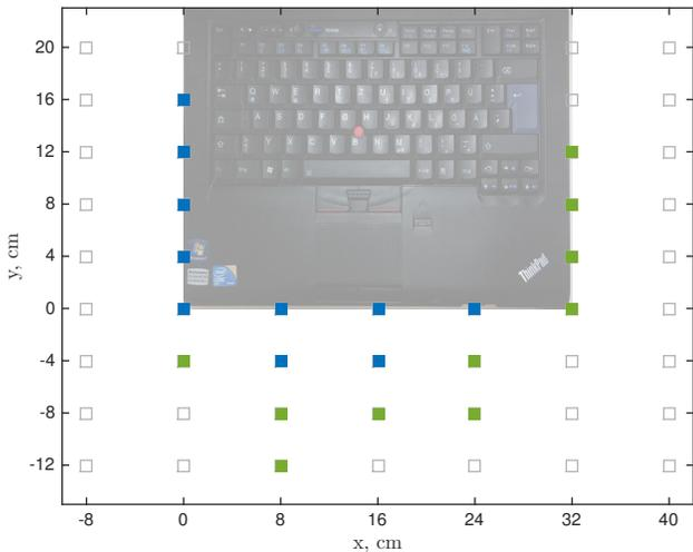
Fig. 6. Presence of the signal. Green marks show a successfully decoded signal using the periodic-based scheme. Blue indicate positions where both encoding schemes are feasible. White marks indicate no detectable signal. We use the following parameters: amplitude modulation:  $t_0 = 0.5s$ , bitrate 2bit/s; periodic-based modulation:  $t_0 = 0.25s$ ,  $t = 15s$ ,  $p_0 = 3$ ,  $p_1 = 5$ , bitrate 0.067bit/s.
